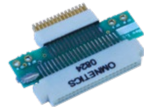
ADPT-HS-36-GMR Input: Omnetics 30 socket Output: Omnetics 44 pin
