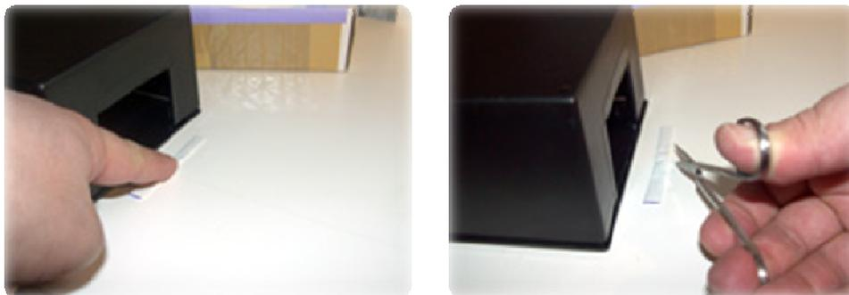
Figure 5-3 Tetrode Wire Placement and Cutting
