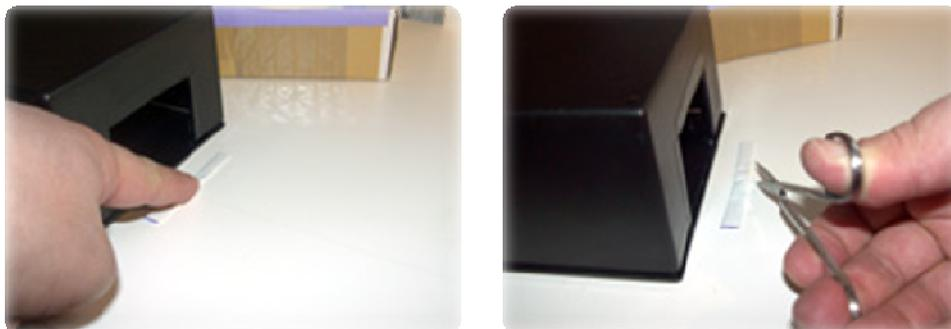
Figure 5-3 Tetrode Wire Placement and Cutting
