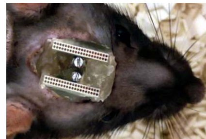
Dual site implant - 2 x 32 channel probes with 2 x nano-Drives
