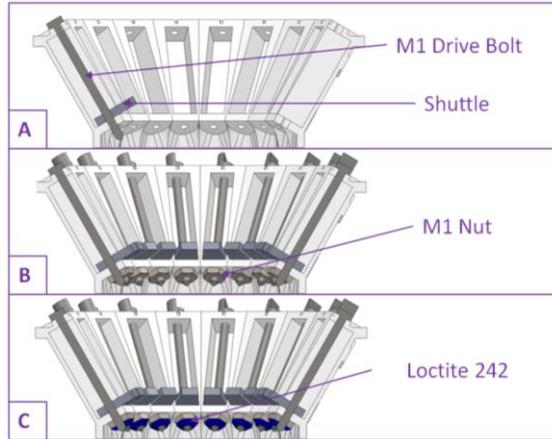
**Figure 4-1 Shuttle Mounting**
