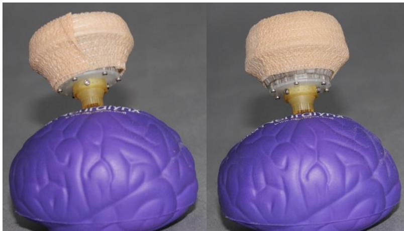
**Figure 6-2 Vetrap Applied to Microdrive Protective Caps**
