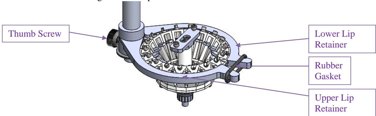
Figure 5-1 Stereotaxic Mount
