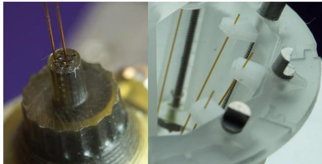
**Figure 4-11 Inserting Polymicro tubing into Microdrive**
