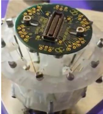
**Figure 4-14 Mounting EIB on top of Microdrive**
