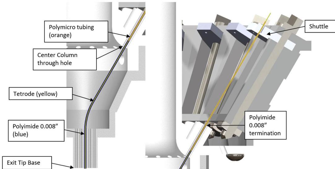
**Figure 4-4 Overview of telescoping Polyimide Polymicro tubing**
