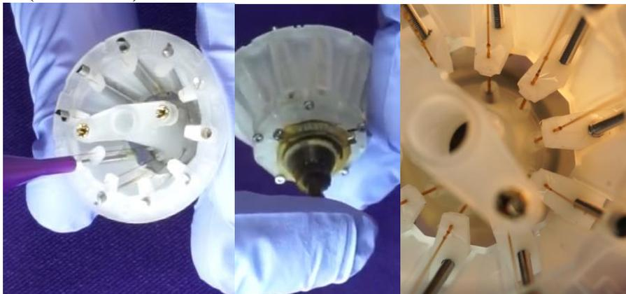
**Figure 4-12 Positioning Shuttles and Polymicro tubing to be secured with epoxy**
