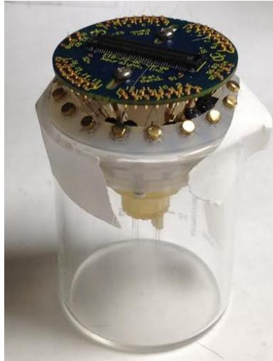
Figure 4-17 Pinned and Fully Assembled Microdrive
