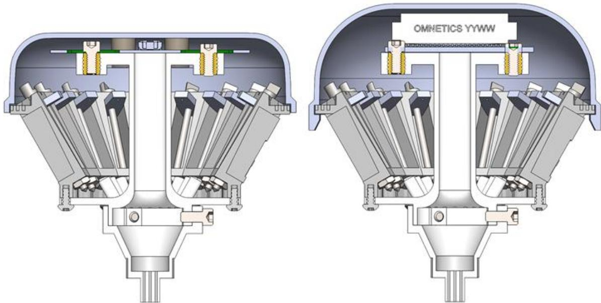
**Figure 6-1 Halo-18 Microdrive QuickClip and Omnetics Protective Cap**
