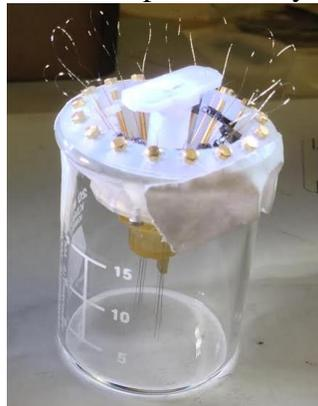
**Figure 4-16 Inserted Tetrodes**
