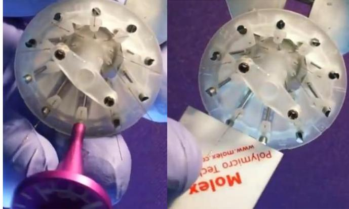
**Figure 4-13 Positioning Shuttles at top of travel and trimming excess Polymicro tubing**
