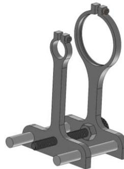
**Figure 2-6 Halo-18 Assembly Jig**
