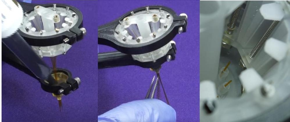
**Figure 4-7 Applying DP-270, advancing Exit tip to Center Column and position Polyimide tubing**
