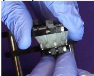
**Figure 4-8 Securing Exit tip to Center Column**
