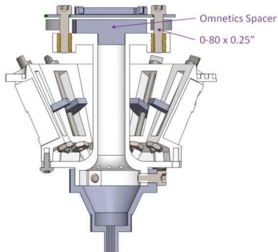
Figure 4-18 EIB-36 Mounted on Halo-10
