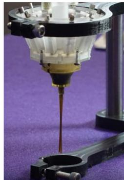
**Figure 4-9 Position of Microdrive and Assembly Jig for curing epoxy**
