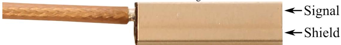
**Figure 7-3 2-Pin BNC Pinout Connections**
