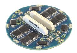
The Neuralynx HS-72-QC is the active electronic part of the headstage (HS) and tether system. It provides 64 channels of unity gain amplification, 8 reference, ground, and 2 differential stimulation lines. The HS-72-QC implements the revolutionary QuickClip<sup>TM</sup> connection method, which allows the HS to self-align and connect to the Electrode Interface Board (EIB) with minimal insertion force.
