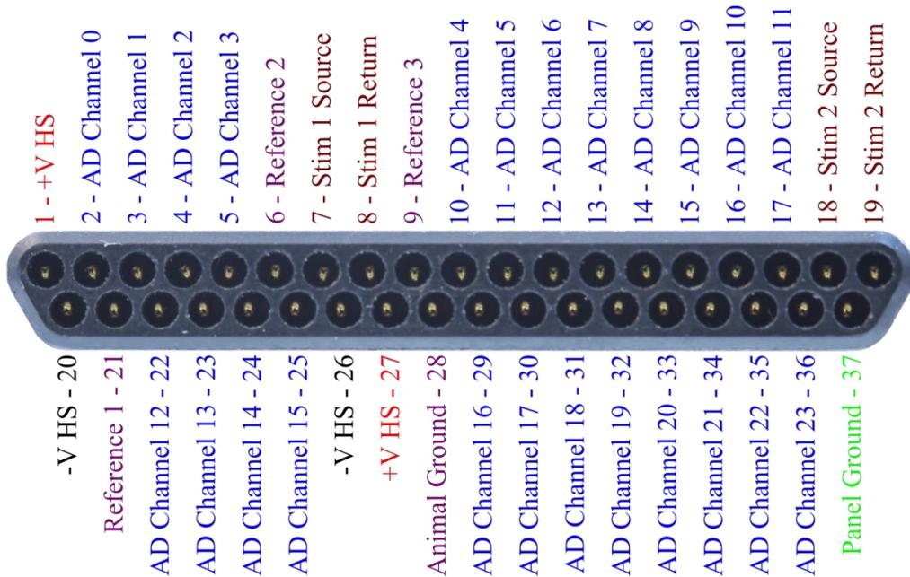
**Figure 1. Pinout of the uDB37 Tether Connector**
