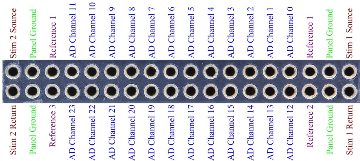
Figure 2. HS-27M Input Connector
