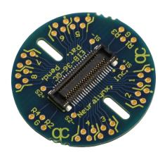
The Electrode Interface Board EIB-36-QC is mounted to microdrive hardware and provides the electronic signal connection between electrode wires and 36 channel Neuralynx Headstage Pre-amplifiers (HS-36-QC). The EIB-36-OC also provides mechanical connection between microdrive hardware and the HS-36-QC.
