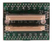
The Electrode Interface Board (EIB-36-16TT) is mounted to microdrive hardware and provides the electronic signal connection between electrode/tetrode wires and two Headstage 36 Pre-amplifiers. The EIB-36-16TT also provides mechanical connection between microdrive hardware and the two HS-36.
