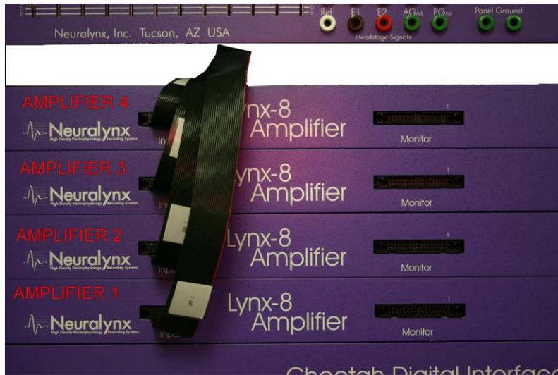
**Figure 5.8 ERP AICA cable AMP# connection**
