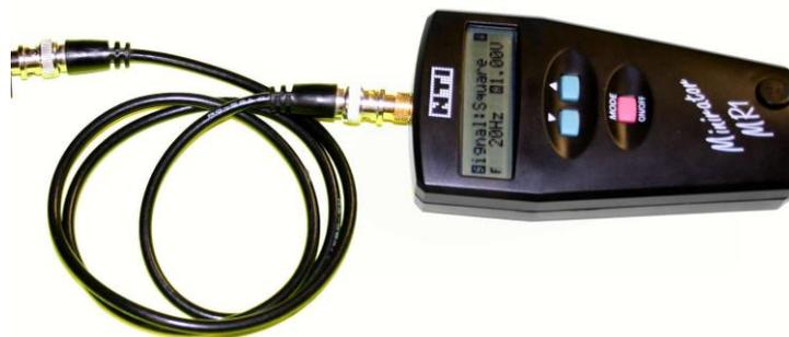
**Figure 7.7 Minirator with BNC cable**
