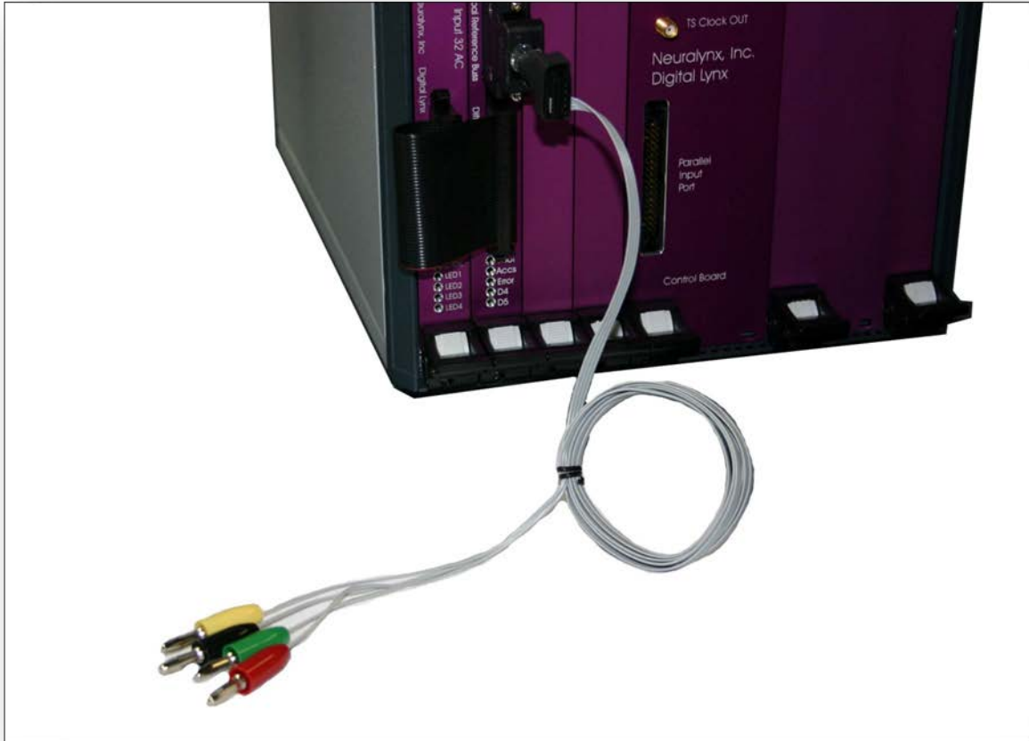
Figure 2 Complete Connection to Digital Lynx
