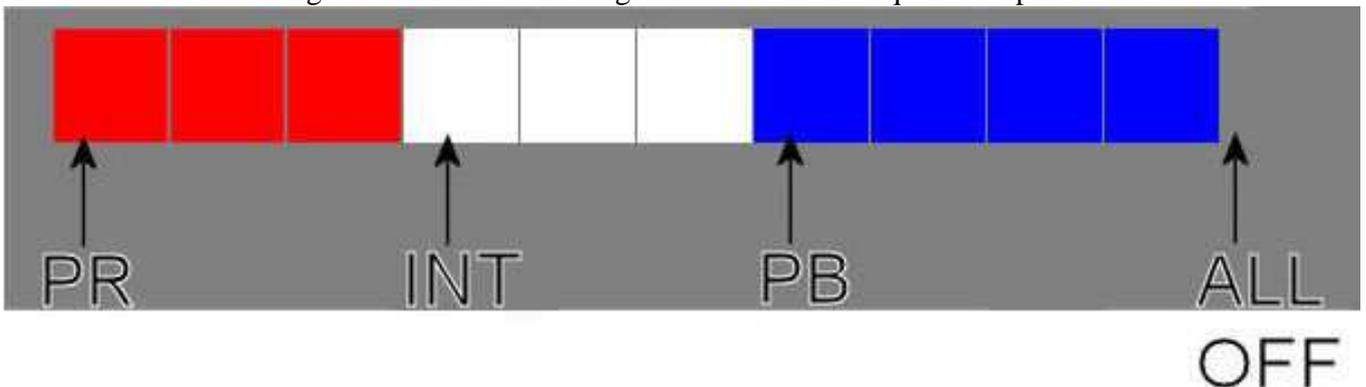
Note that the PureRed transitions OFF at the first whitepixel and Intensity transitions off at the first blue pixel (where PureBlue transitions ON). Cheetah 5 and newer also has a built in noise filter that ignores transitions that do not last long enough to be considered a trackable object.
