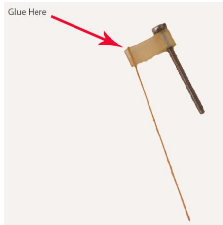
Figure 12-1 Installing the Polymicro Tubing
