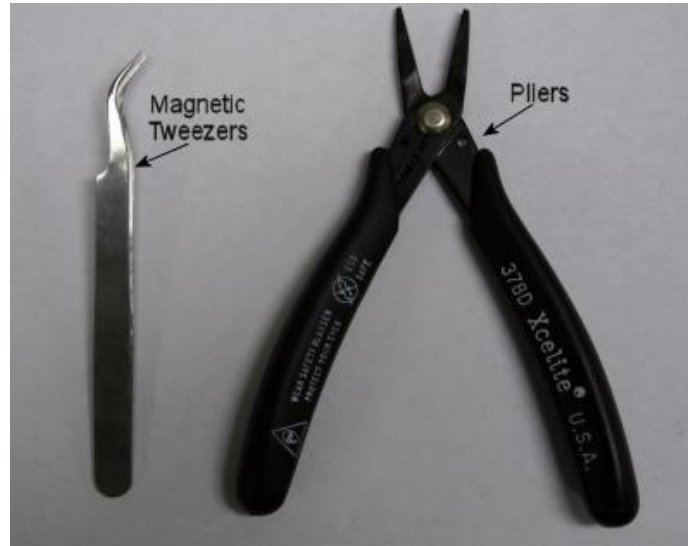
Figure 17-4 EIB Pinning Tools
