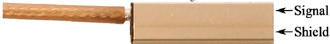
Figure 6-3 2-Pin BNC Pinout Connections
