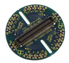
The Electrode Interface Board EIB-72-OC-Small is mounted to microdrive hardware and provides the electronic signal connection between electrode wires and 72 channel Neuralynx Headstage Pre-amplifiers (HS-72-QC). The EIB-72-QC-Small also provides mechanical connection between microdrive hardware and the HS-72-OC.
