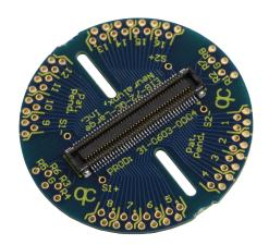
The Electrode Interface Board EIB-72-QC-Large is mounted to microdrive hardware and provides the electronic signal connection between electrode wires and 72 channel Neuralynx Headstage Pre-amplifiers (HS-72-QC). The EIB-72-QC-Large also provides mechanical connection between microdrive hardware and the HS-72-QC.
