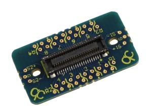
The Electrode Interface Board EIB-36-QC-Simple is mounted to microdrive hardware and provides the electronic signal connection between electrode wires and 36 channel Neuralynx Headstage Pre-amplifiers (HS-36-QC). The EIB-36-QC-Simple also provides mechanical connection between microdrive hardware and the HS-36-QC.
