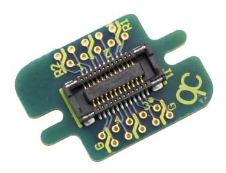
The Electrode Interface Board EIB-16-QC-H is primarily designed for use with the Harlan 4 microdrive. Its unique lightweight design allows for direct access to all drive screws. This EIB is mounted to the Harlan Drive and provides the electronic signal connection between electrode wires and a 16 channel Neuralynx Headstage Pre-amplifiers (HS-16-QC). The EIB-16-QC-H also provides mechanical connection between microdrive hardware and the HS-16-QC.
