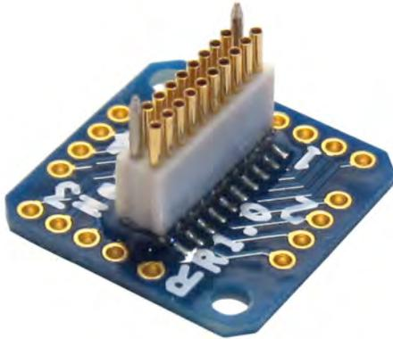
The Electrode Interface Board EIB-16-F is designed primarily to hold a NLX-5 or Harlan 4 microdrive in place during microdrive installation. It can also be utilized as a holder when affixing a Neuralynx EIB-8, EIB-16, or EIB-18 to a subject.
